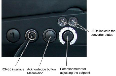
Using the potentiometer, the current setpoint value can be increased or decreased. A malfunction can be acknowledged by pressing the Acknowledgement button. A red LED indicates a malfunction.
